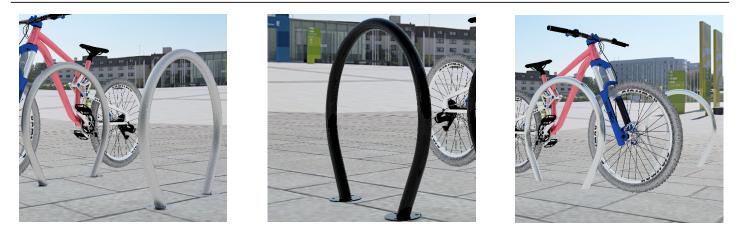
The VELOPA Catthorpe Cycle Stand is a shaped tubular cycle stand. The design allows the frame of the bicycle to be secured by the users own security lock. The Catthorpe Stand is suitable for securing two bicycles. Available in galvanised steel, galvanised and coated and grade 304 stainless steel, with ragged feet for casting into new concrete or flanged feet for bolting to an existing surface.
