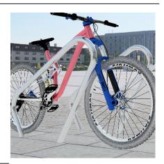
The VELOPA Lilbourne Cycle Stand is a shaped tubular cycle stand. The design allows the frame of the bicycle to be secured by the users own security lock. The Lilbourne Cycle Stand is suitable for securing two bicycles. Available in galvanised steel, galvanised & coated or grade 304 stainless steel, with ragged feet for casting into new concrete or flanged feet for bolting to an existing surface.
