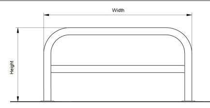
Perimeter Barriers are designed to help secure site perimeters and provide a permanent obstacle to vehicle access, to mark boundaries, define trolley parks and protect vulnerable door entrances and exits.
