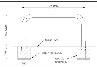
Key Locking Removable Perimeter Barriers are designed to help secure site perimeters and provide a permanent obstacle to vehicle access. Best suited to sites where aesthetics, security and flexibility are equally important.
