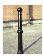
The AUTOPA Exeter Polyurethane Bollard has a traditional design and offers site owners a robust vehicle access control solution. Corrosion and shatter proof, this bollard is cast in an engineering grade, heavy duty polymer around a steel core and is ideal for use around parking areas, pavements and pedestrianisation schemes.
