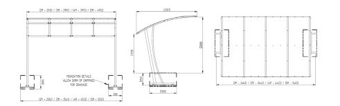
The VELOPA Banbury Cycle Shelter is a fully modular, contemporary, cantilevered cycle shelter. Manufactured from galvanised mild steel as standard to ensure its longevity, the Banbury Shelter is compatible with all standard height VELOPA cycle stands and racks. Complete with 4mm UV stabilised PETG clear sheet roof.
