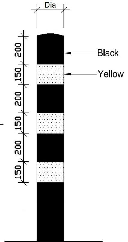
The AUTOPA range of Black & Yellow bollards are ideal for providing high visibility protection in both internal and external warehousing environments. All products in the range are galvanised mild steel, ensuring their longevity and are designed to take the knocks and bumps that occur in all warehouse environments.
