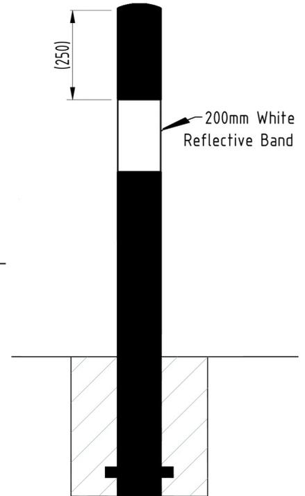
The AUTOPA range of Black & White bollards are ideal for providing high visibility protection in both internal and external warehousing environments. All products in the range are galvanised mild steel, ensuring their longevity and are designed to take the knocks and bumps that occur in all warehouse environments.
