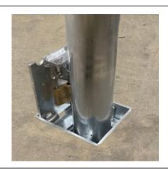
The Removable Bollard offers an effective, simple and robust way to protect premises and vehicles. Removable Bollards are particularly suitable for locations where occasional access is required, the simple tab and padlock system provides an easy to operate solution for locking the bollard in place. The Removable Bollard is 1,000mm above ground and is available in a range of outside tube diameter sizes from 60mm through to 219mm. Padlock to secure is available at an extra cost.
