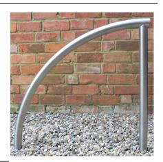
The Duston Cycle Stand is a shaped tubular cycle stand. The design allows the frame of the bicycle to be secured by the users own security lock. The Duston Cycle Stand is suitable for securing two bicycles. The Duston Cycle Stand is available in galvanised steel, galvanised & coated or grade 304 Stainless Steel, with ragged feet for casting into new concrete or flanged feet for bolting to an existing surface.
