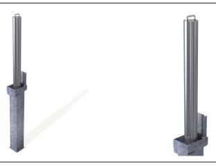
The RetractaPost-GL offers a highly effective and robust way to protect premises and vehicles. The RetractaPost-GL is raised and lowered vertically and is 900mm tall when raised. When lowered the post is fully below ground and covered using the integral lid. The post is lockable in the raised position by rotating the post 45° and then pressing the high-security push button 7-pin security lock. The post is unlocked using the supplied key, rotated and then lowered.
