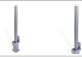
The RGP (Removable Ground Post) offers a highly effective and robust way to protect premises and vehicles. The post is 900mm above ground, when removed the socket is covered using the integral lid. The post is lockable by rotating the post 45° and then pressing the high-security push button 7-pin security lock. The post is unlocked using the supplied key, rotated and then removed.
