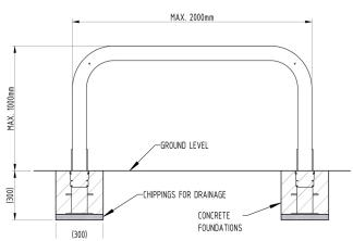
Key Locking Removable Perimeter Barriers are designed to help secure site perimeters and provide a permanent obstacle to vehicle access. Best suited to sites where aesthetics, security and flexibility are equally important.
