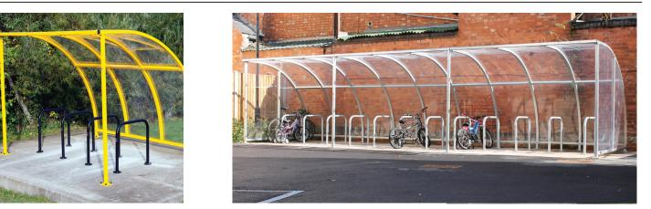
The Stratford shelter is a free-standing, single sided cycle shelter designed for on site assembly, constructed from galvanised steel and PET sheet. The frame is made from 50mm galvanised mild steel square tube. The roof is 4mm clear sheet.
