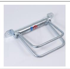
The simplest cycle holder, a familiar sight throughout the UK, allows the tyre of the bicycle to be supported. The stand is fixed to a suitable wall and can be spaced at not less than 610mm between holders for cost effective cycle parking. The Model R is available in either 90° or 45° versions which allow for cycles to be parked either head-on or angled.
