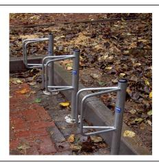
The Model SU (V) is a freestanding variant of the simplest cycle holder, the Model R. A familiar sight throughout the uk, these holders allow the tyre of the bicycle to be supported. the Model SR (V) is a suitable for two bicycles. The stand is fixed to the ground, in either concrete in or bolting down versions and can be spaced at 610mm apart for cost effective cycle parking.
