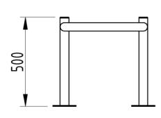
Functional and robust in design, AUTOPA's range of column protectors are designed to protect corners, columns, and other vulnerable pillars from vehicle damage in a busy industrial environment. Our Column Protectors are manufactured from mild steel and galvanised to ensure their longevity. Suitable for both internal and external use.
